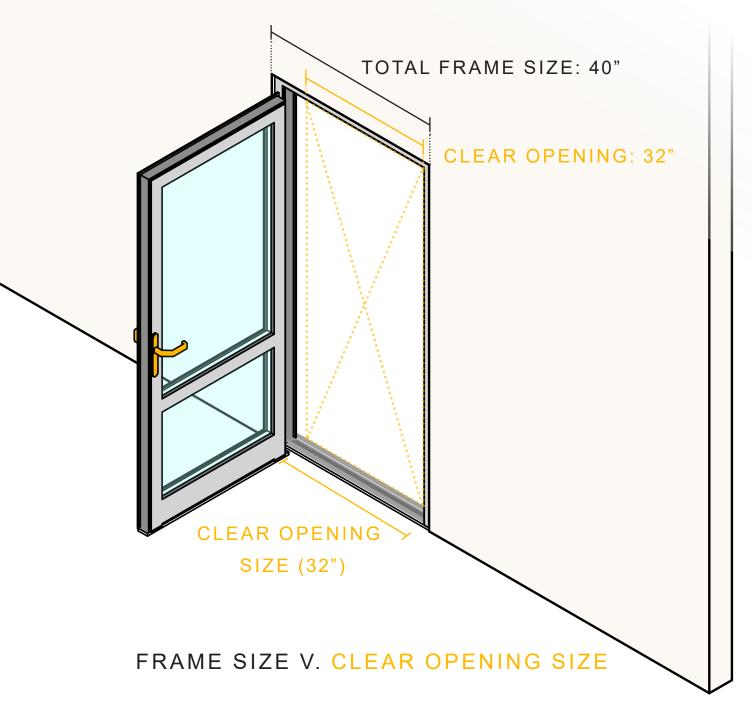
This is an important distinction for sizing doors. For example, a 40" frame will have roughly a 32" clear opening. The FRAME SIZE accounts for the total frame fitted to the rough opening. The CLEAR SIZE measures the acutal opening size, which subtracts the size of the frame and the thickness of the open door itself. For comparison, a traditionally sized 36" wood door would have a 32" clear because the frame itself is much smaller and less energy efficient.
